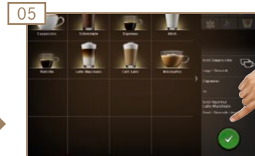
05 Start preparation of each of the products in the waiting list by pressing the green button. The outlet moves down. Next preparation begins.
